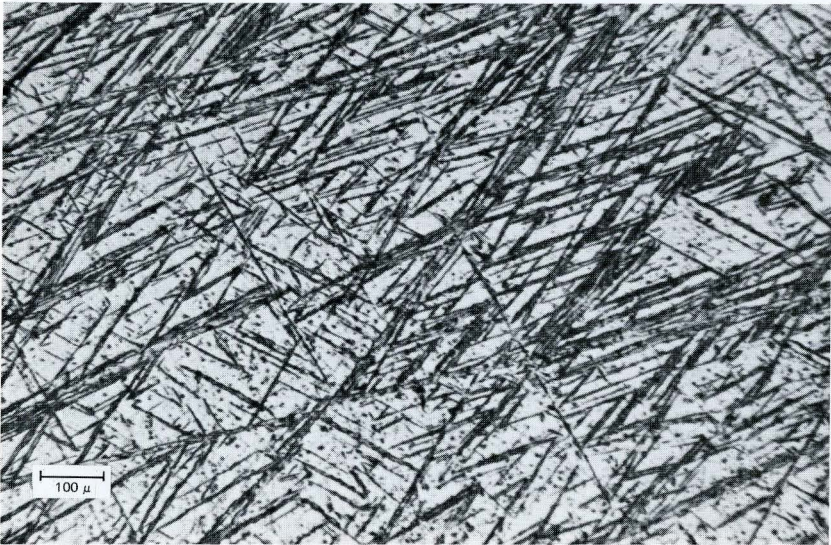
Fig. 4 Feathering and multiplication of Neumann bands in kamacite
