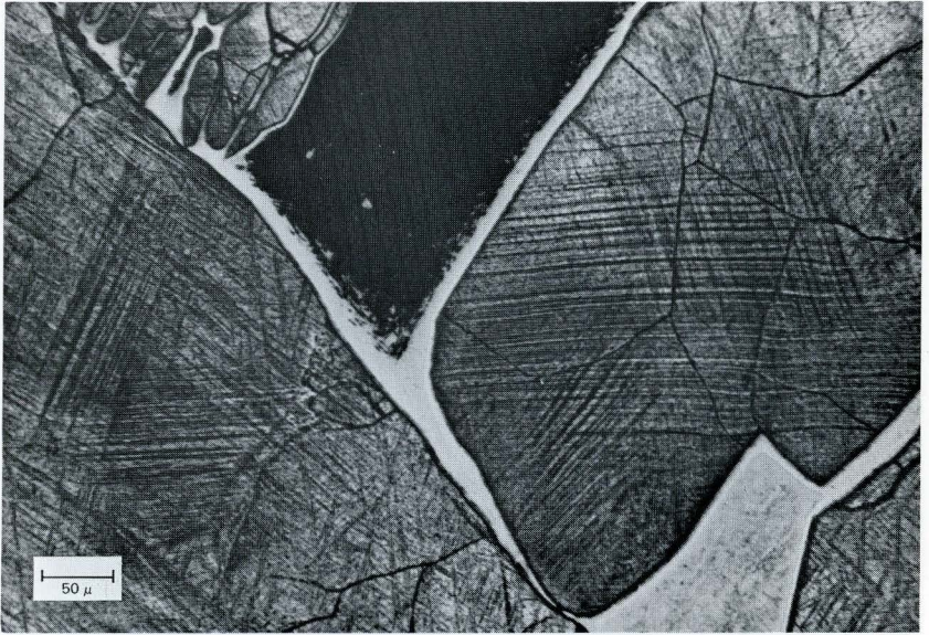
Fig. 5 Hatched pattern in kamacite indicating shock intensity in the 600 kb range. The light area is taenite and the dark area (top center) is a plessite field.
