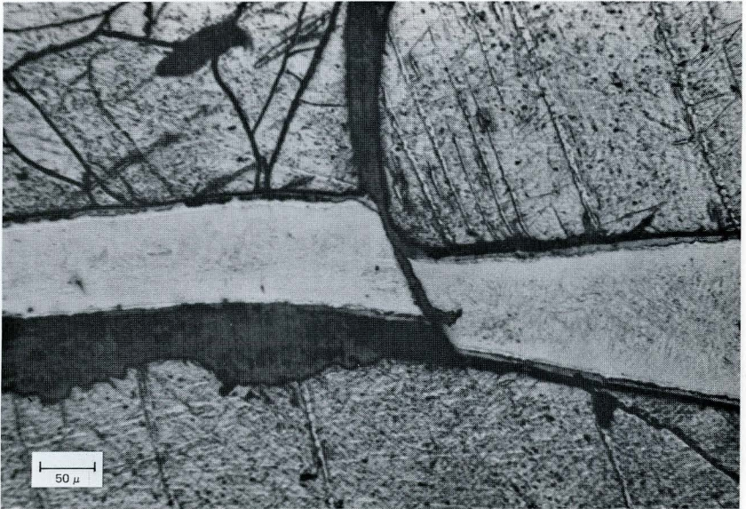
Fig. 6 Offset taenite band with oxidized material running along and through it
