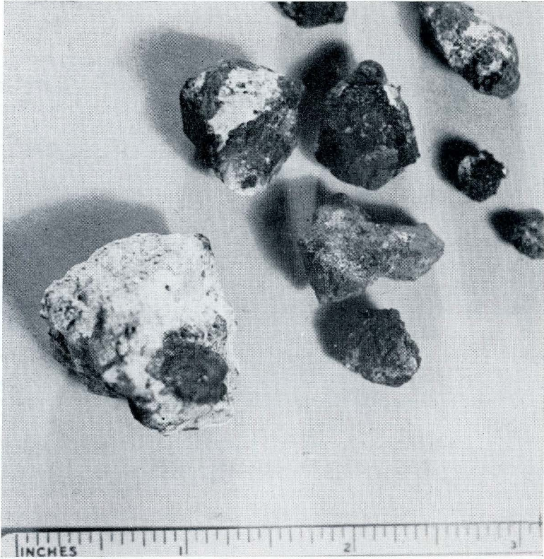
FIG. 3. Collection of nickel-iron inclusions.
