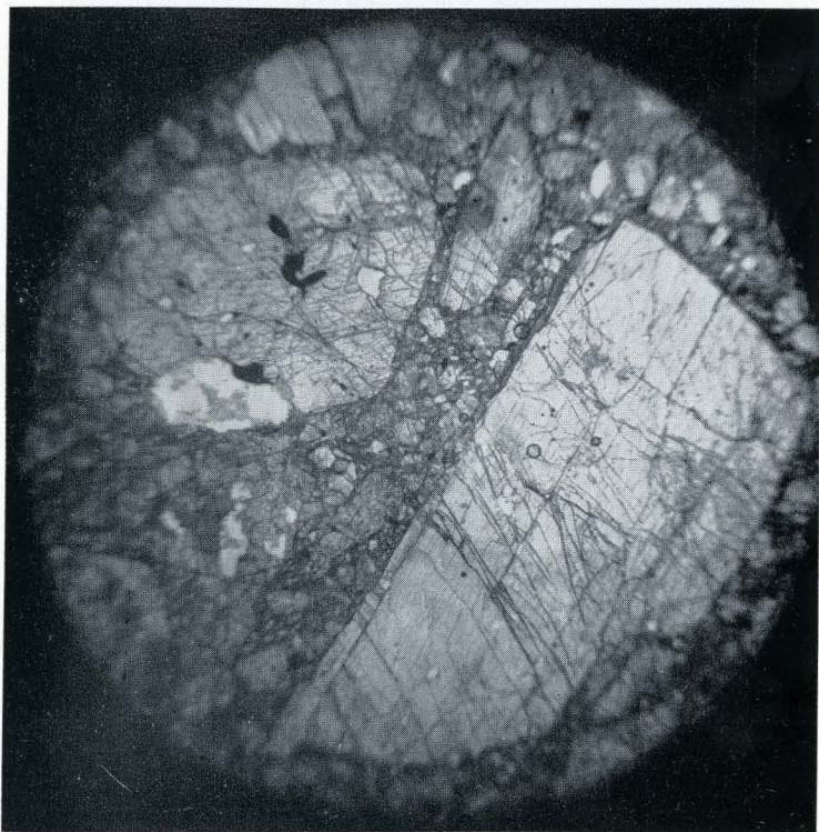
FIG. 4. Photomicrograph of well-developed enstatite crystals. \times 200 .
