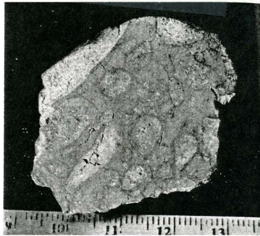
Fig. 3. Cut surface of NWA 5782 showing its brecciated texture. Units on scale (rule) are in cm ches.
