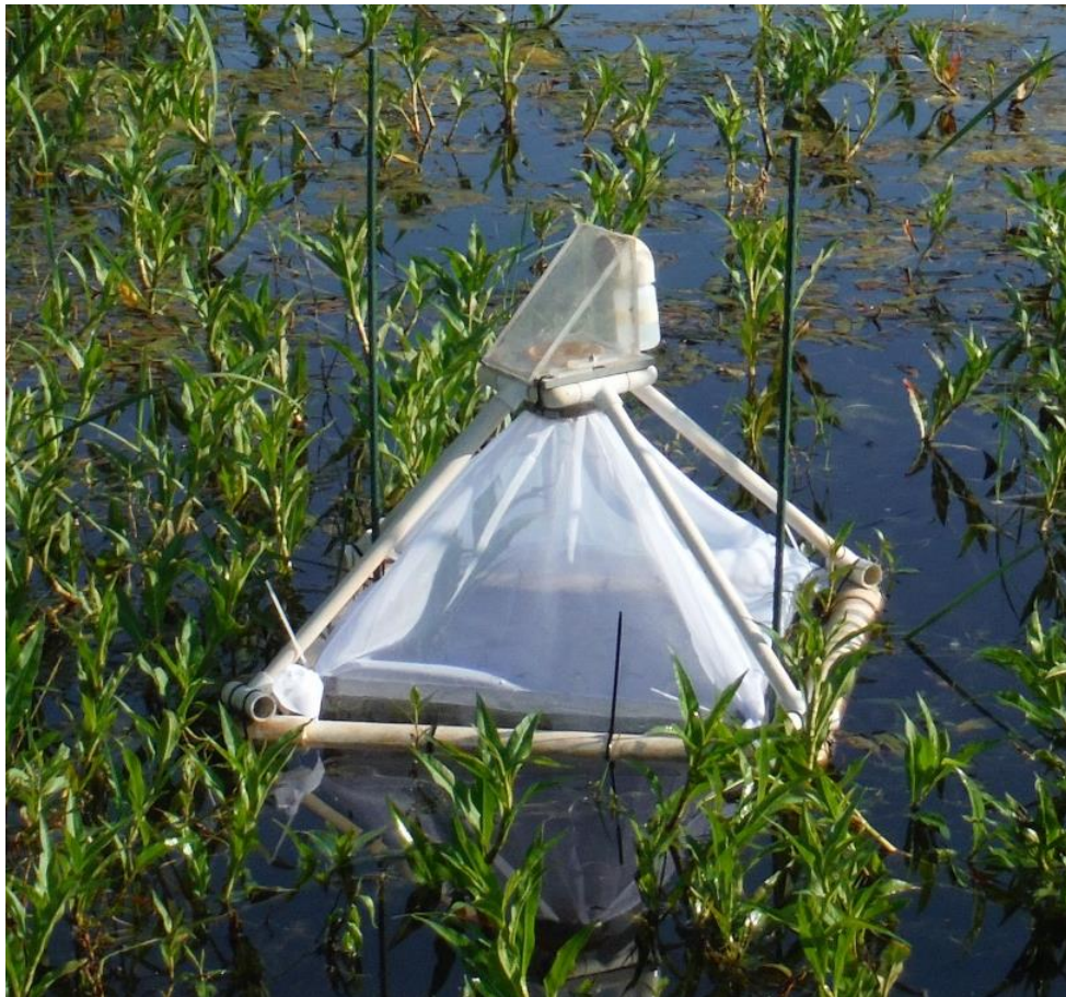
Figure 1: Pyramid-shaped floating emergence trap used to sample adult emerging insects, secured with 1-cm diameter plastic-coated stakes.
