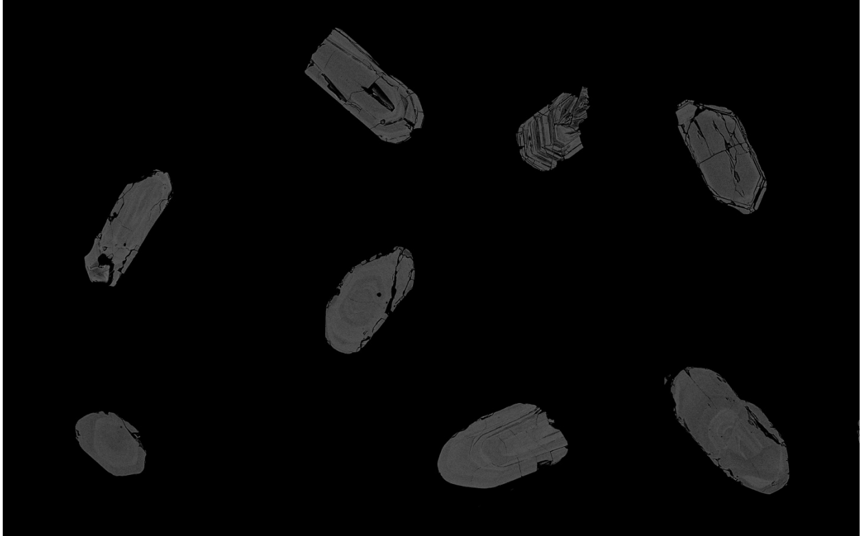
Figure 14. Selected backscattered electron image of zircon concentrations from BW3 (Carter Sandstone) that was used for detrital zircon geochronology.
