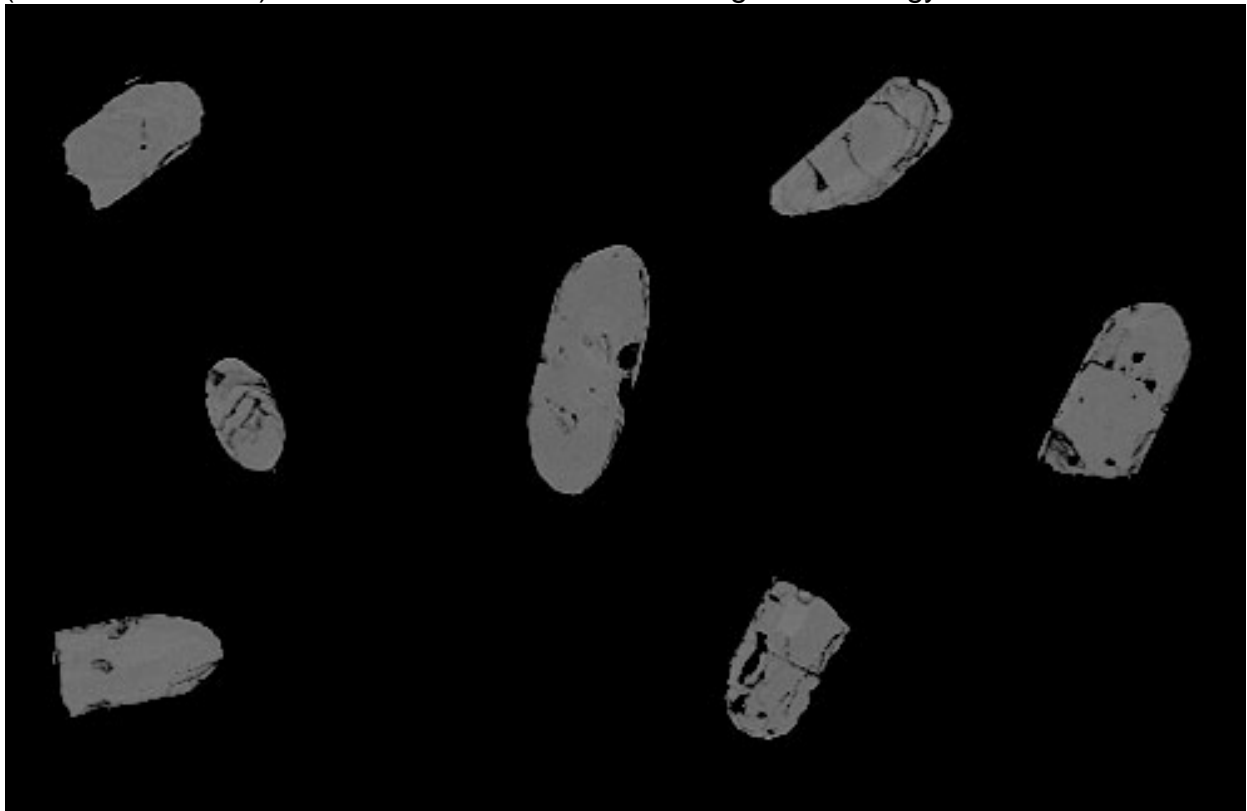
Figure 13. Selected backscattered electron image of zircon concentrations from BW2 (Sanders Sandstone) that was used for detrital zircon geochronology.
