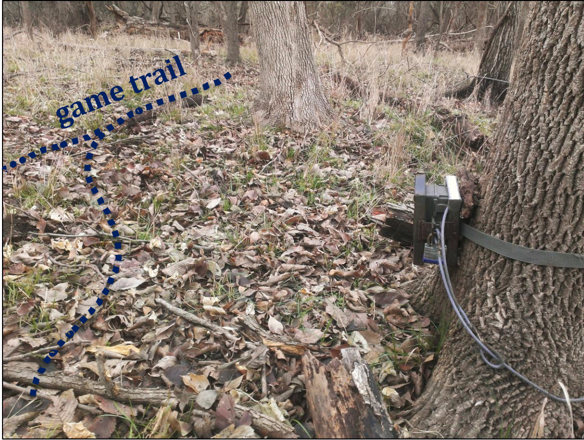
Figure 4. A representation of how we set up a digital game camera trap station to face perpendicular to a game trail approximately two meters away from the mounting structure and camera. In this photograph, we added dashed lines to clarify the game trail pathway.
