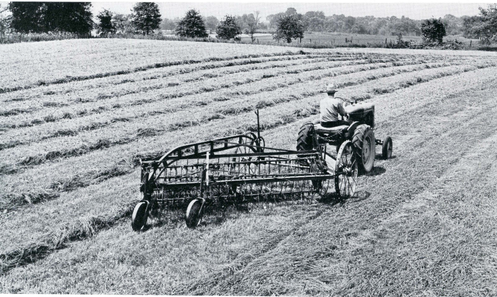
This side delivery rake with tedding features provides clean, continuous raking action.
