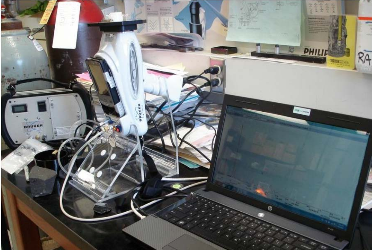
Figure 2.3 – Bruker handheld Tracer IV benchtop setup. From Conrey and Wolff (2011).
