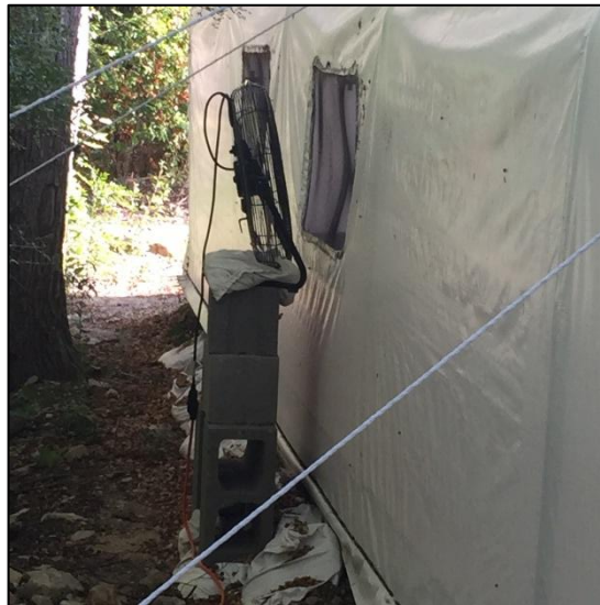
Figure 5. A 20-in HDX high-velocity floor fan on concrete cinder blocks was used to circulate air throughout the flight facility.
