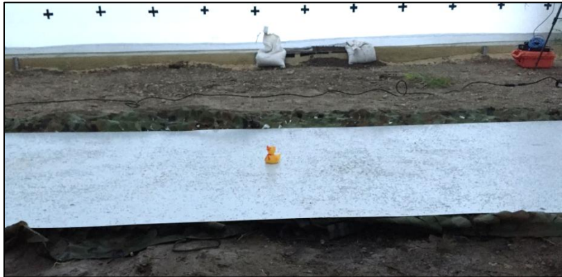
Figure 20. Image showing rubber duck used to focus the high-speed IL4 camera on the center of a treatment surface.
