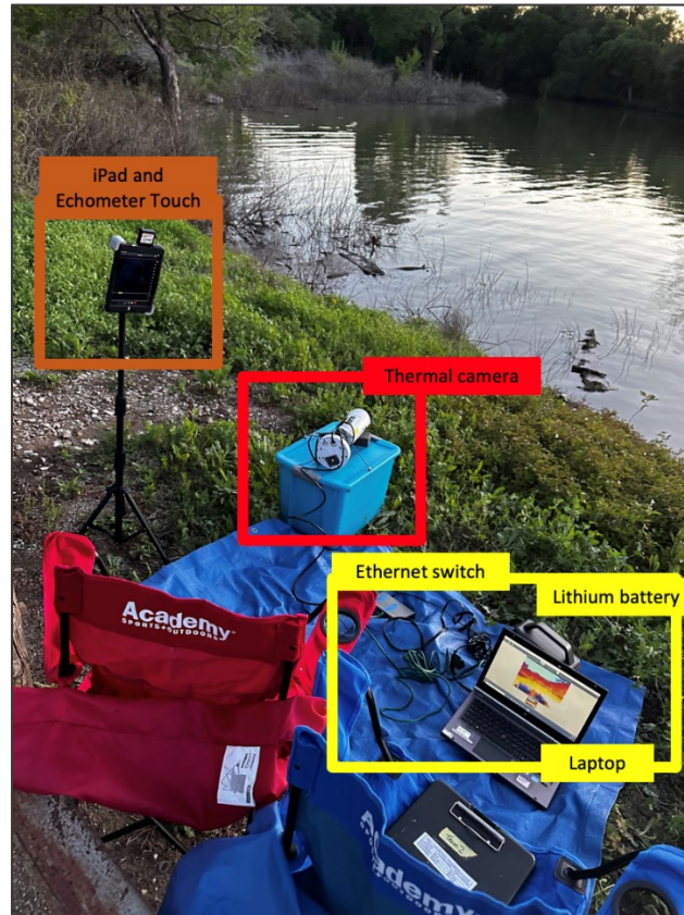
Figure 2: Annotated picture of equipment set-up used in thermal and acoustic monitoring surveys conducted between 2021 to 2024 in Fort Worth, Tarrant County, Texas, USA.
