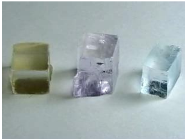
Figure 2.1: NaCl, KCl, and KBr after irradiation with a Tesla coil 79 , showing presence of color centers.
