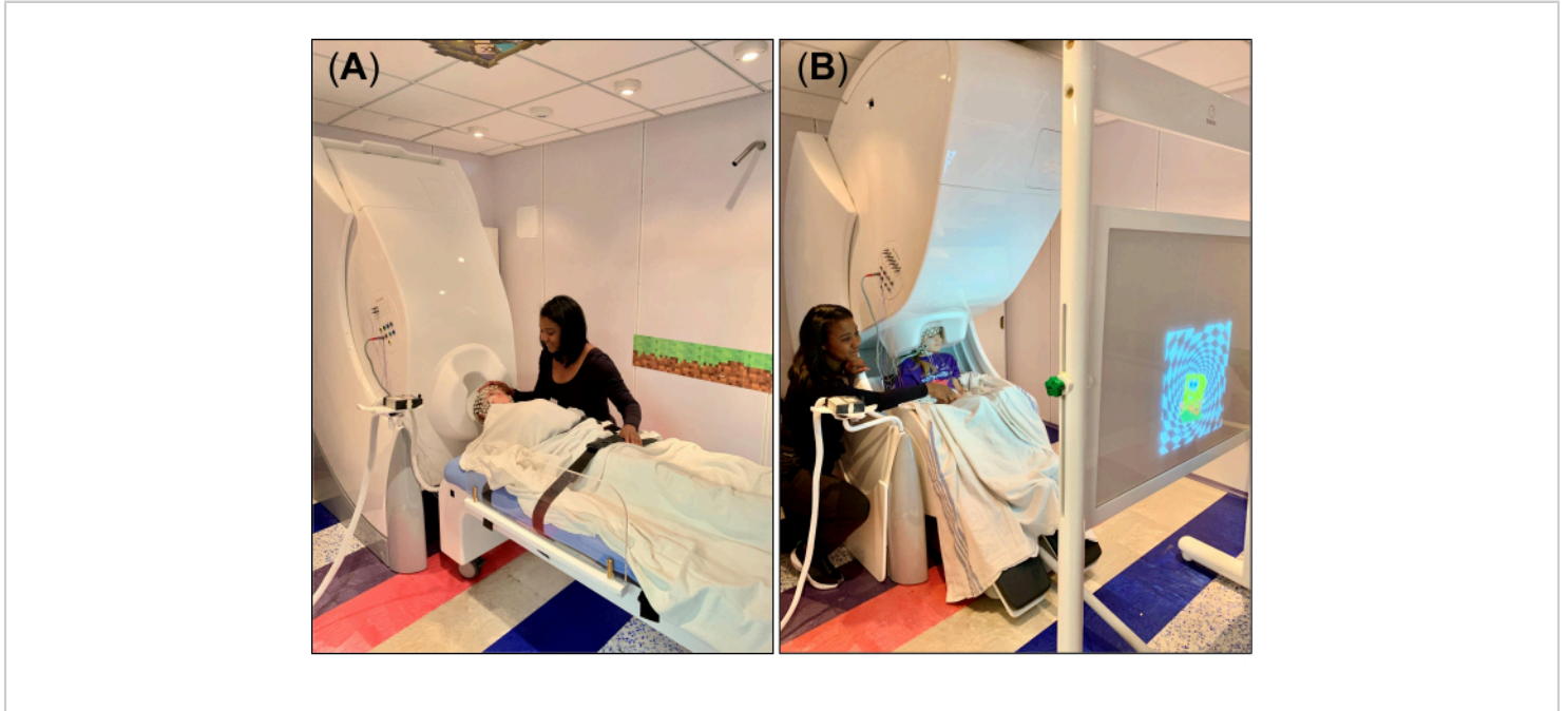
Figure 1: Experimental setup for simultaneous MEG and HD-EEG at CCHCS. (A) HD-EEG (256 channels) and MEG (306 sensors) systems with the gantry of the MEG set to a supine position (90°, horizontal position) for a resting/sleeping state recording using the nonmagnetic MEG-compatible bed. The technician is preparing the subject (a 9-year-old girl) for the recording while ensuring safety and comfort. (B) HD-EEG and MEG systems set for a recording in a seated position using the nonmagnetic MEG-compatible chair. The technician is preparing the subject for the recording while ensuring the correct position of the subject in front of the screen where visual stimuli will be projected during the visuomotor task. Please click here to view a larger version of this figure.
