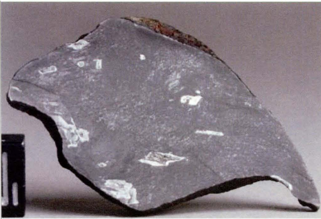
Polished and etched internal surface of shrapnels showing schreibersite inclusions
