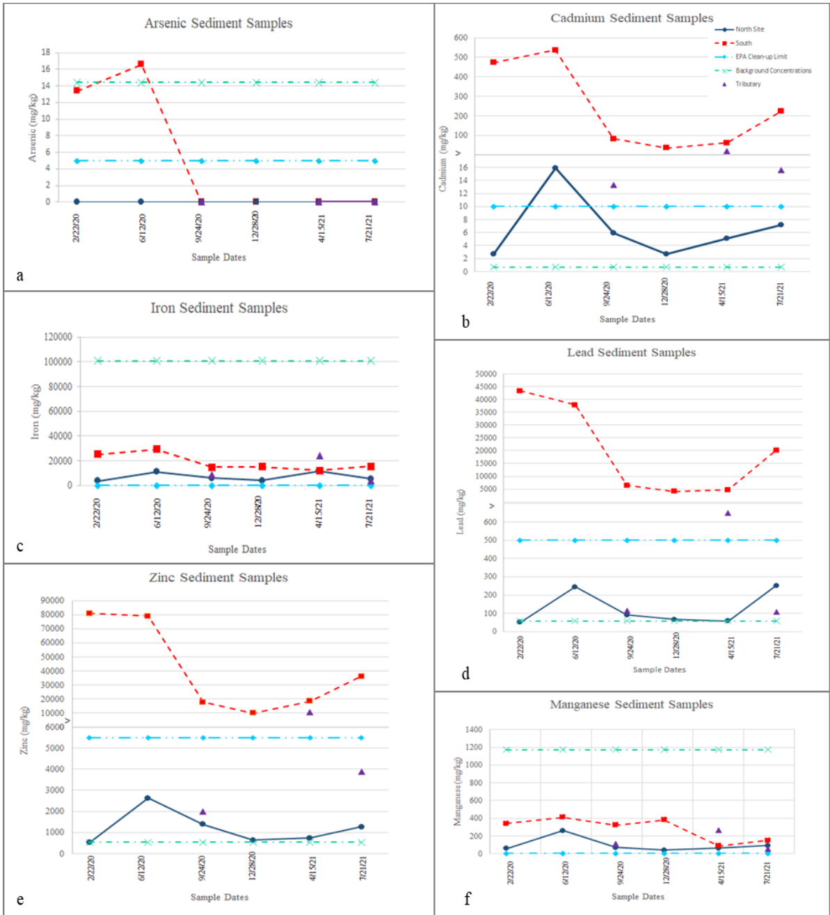
Figure 8: Sediment metal analysis: a. Arsenic, b. Cadmium, c. Iron, d. Lead, e. Zinc, and f. Manganese. Dark blue line indicates changes at north location, red line indicates changes at south location, turquoise line indicates EPA clean-up standard, green line indicates background concentrations, and the tributary samples are indicated by a purple triangle.
