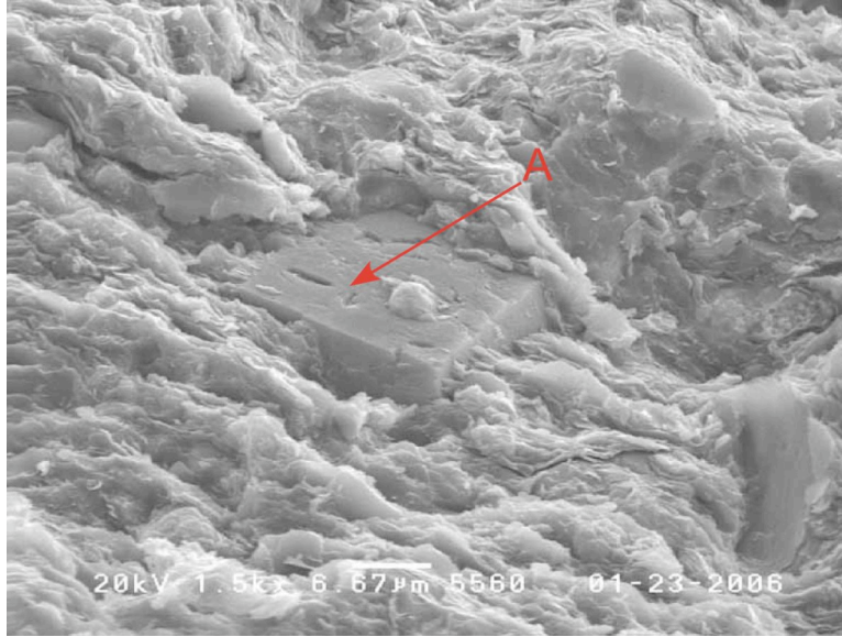
Figure IV. 5. Ross Draw Unit #5, lower Barnett interval C, 15,560 feet–15,570 feet (magnification 1500x). Kaolinite clay matrix with dolomite rhomb (A).
