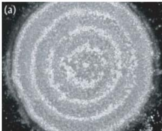
Figure 7. Optical micrograph illustrating circular calcium phosphate patterns (0.9 mm diameter) on silicon formed by using an automated spark-ablation apparatus. Taken from reference 82.
