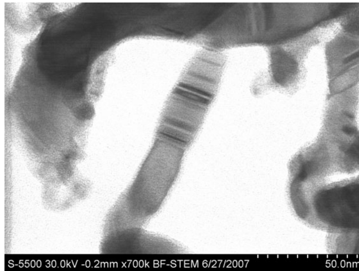
Figure 4.12: SiC nanowires produced after 8 hours sintering are shown in this HRSEM image of Sample TFA8. Striping indicates stacking faults in the crystal structure inside solid nanowires.
