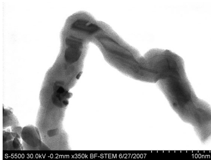
Figure 4.19: In this HRSEM image, Sample TFA3 shows clear crystalline structure inside the SiC nanowires.
