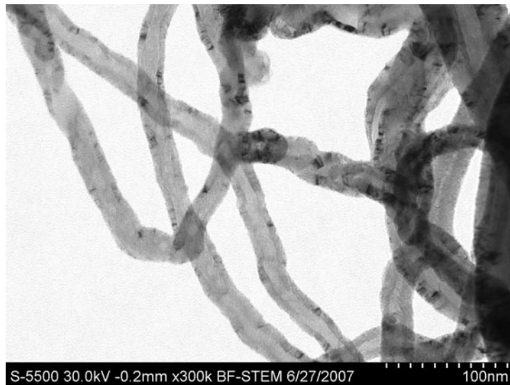
Figure 4.6: HRSEM image of tube furnace sample TFA1 sintered for 1 hour at 1200°C.
