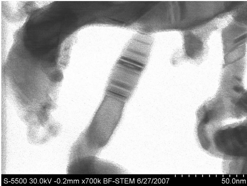
Figure 5.11: HRSEM image of TFA8 shows stacking faults inside the SiC nanowire and an amorphous surface layer about 1 nm thick.
