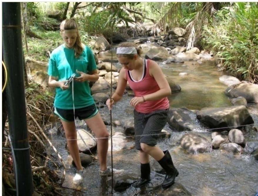
Figure 10: Taking cross-sectional data at study site 2.
