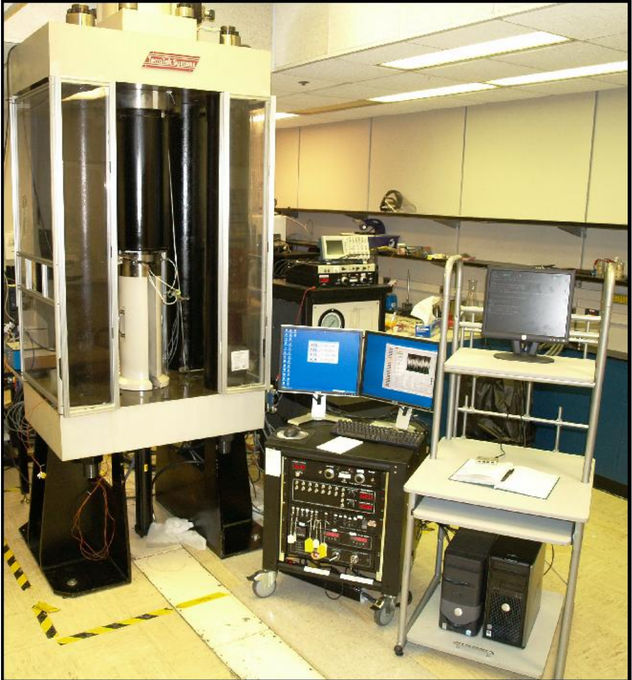
Figure 15. TerraTek 375 ton stiff loading system used for the experiment.
