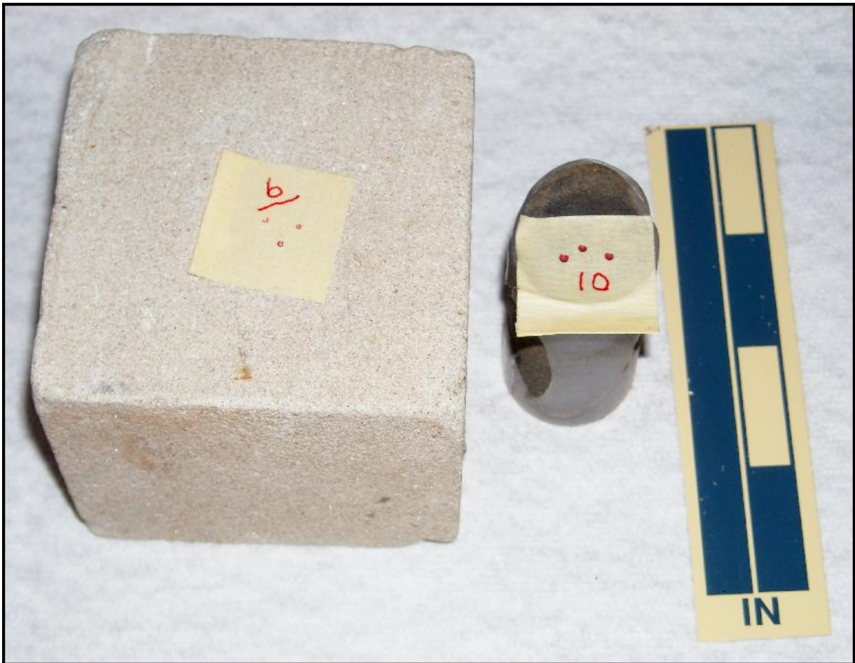
Figure 19. Berea Sandstone Dimple test of companion block and test sample. Dimple diameters of 6 and 10 ticks, respectively. The color darkening and larger Dimple diameter on the test sample is due to the exposure to hydraulic fluid.
