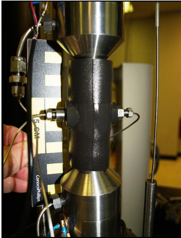
Figure 17b. Radial flow-through Hassler coreholder positioned in the triaxial compression loading configuration.
