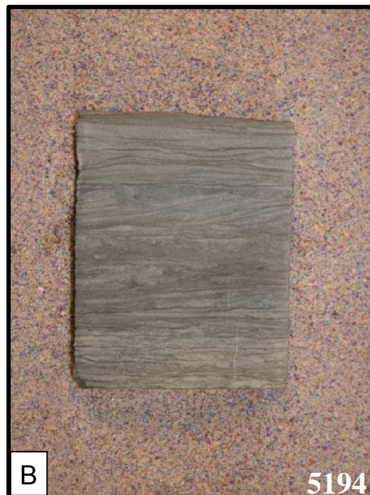
Figure 30. Core photos of facies D. Photo A shows highly bioturbated light gray siltstone. Photo B shows laminae within light gray siltstone. Core is 8 cm wide.
