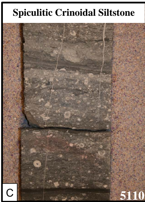
Figure 18. Core photos of lithologies present in the House No. 1 well. In this and following core photographs, white numbers in lower right corner indicate depth (in ft.) at which core was taken. Core is 8 cm wide.
