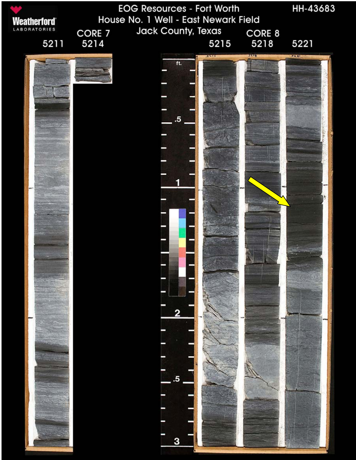
5211 - 5224 ft. Facies C and E. Note thin, laminated claystone interval of facies E (yellow arrow) interbedded with facies C.
