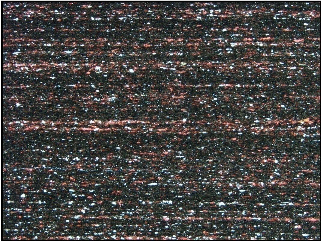
Figure 33. Photomicrograph of distinct laminae within facies E. Plane-polarized light. FOV is 10.25 mm across. Depth in core is 5,281.4 feet.
