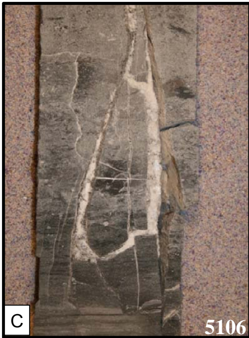
Figure 38. Core photos of fractures in Marble Falls clastic interval. Photo A and B are of facies A. Photo C is of facies B. Photo D is of facies G. Core is 8 cm wide.
