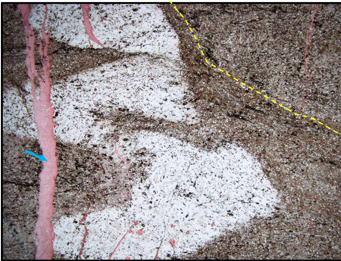
Figure 24. Photomicrograph of burrow in facies A. Lamination (yellow line) in matrix is bent around burrow. Vertical fracture cutting burrow is completely healed mostly by calcite and some dolomite. Plane-polarized light. FOV is 29 mm across. Depth in core is 5,064.5 feet.
