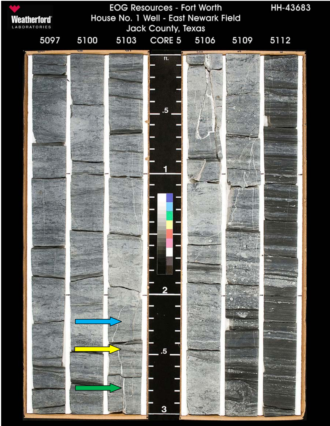
5097 - 5115 ft. Facies A and B. Note gradational contact (yellow arrow) between facies A (blue arrow) and facies B (green arrow). Also note interbedded crinoidal siltstone in black laminated claystone with fracturing.
