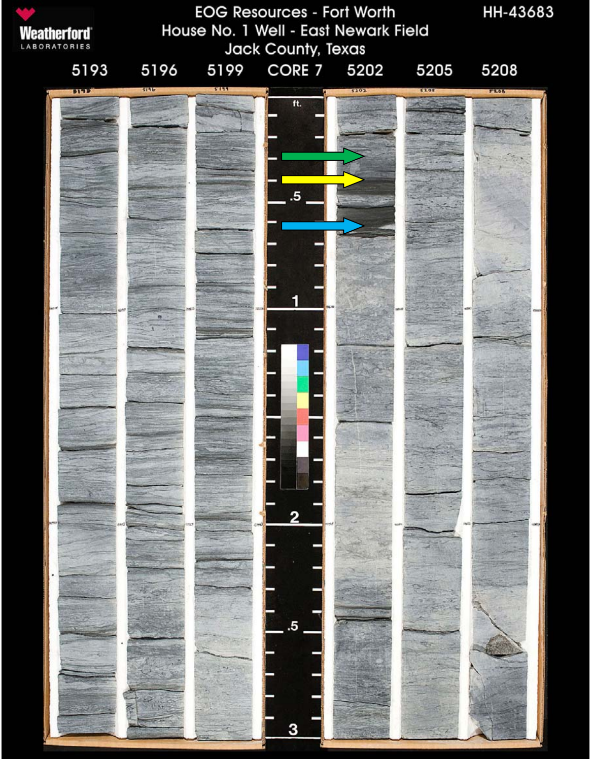
5193 - 5211 ft. Facies D and C. Note sharp contact (yellow arrow) between facies D (green arrow) and C (blue arrow).
