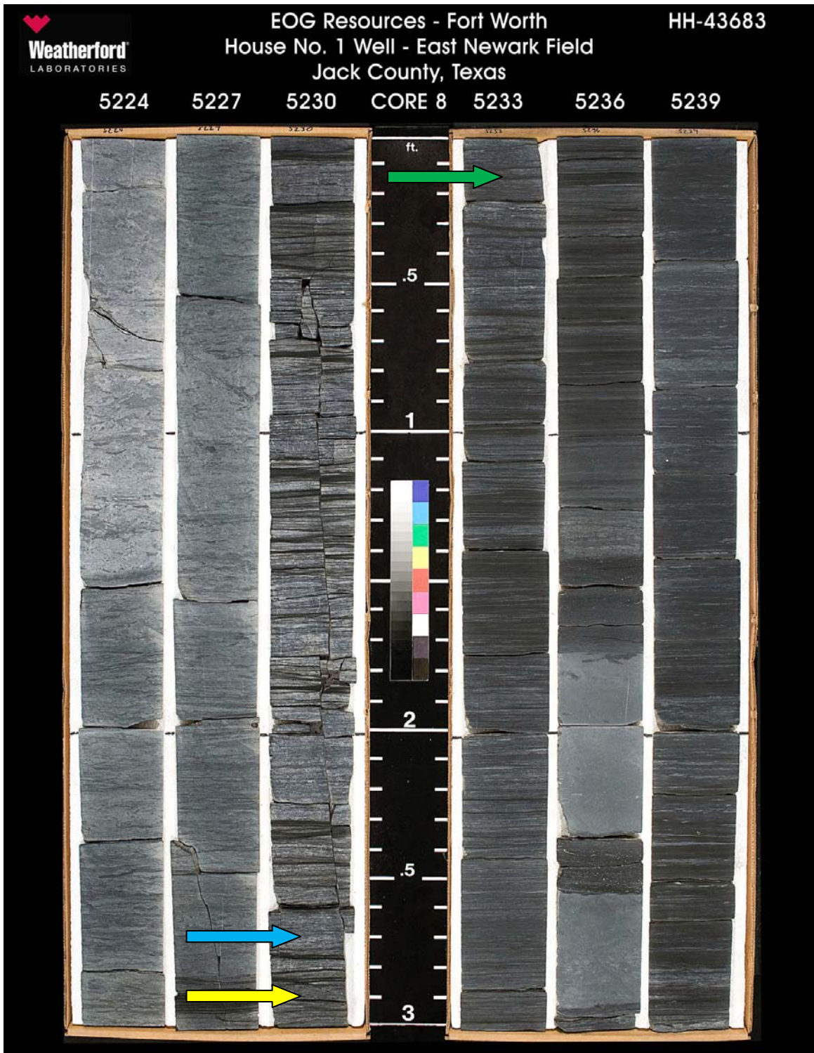
5224 - 5242 ft. Facies C and D. Note gradational contact (yellow arrow) between facies C (blue arrow) and E (green arrow).
