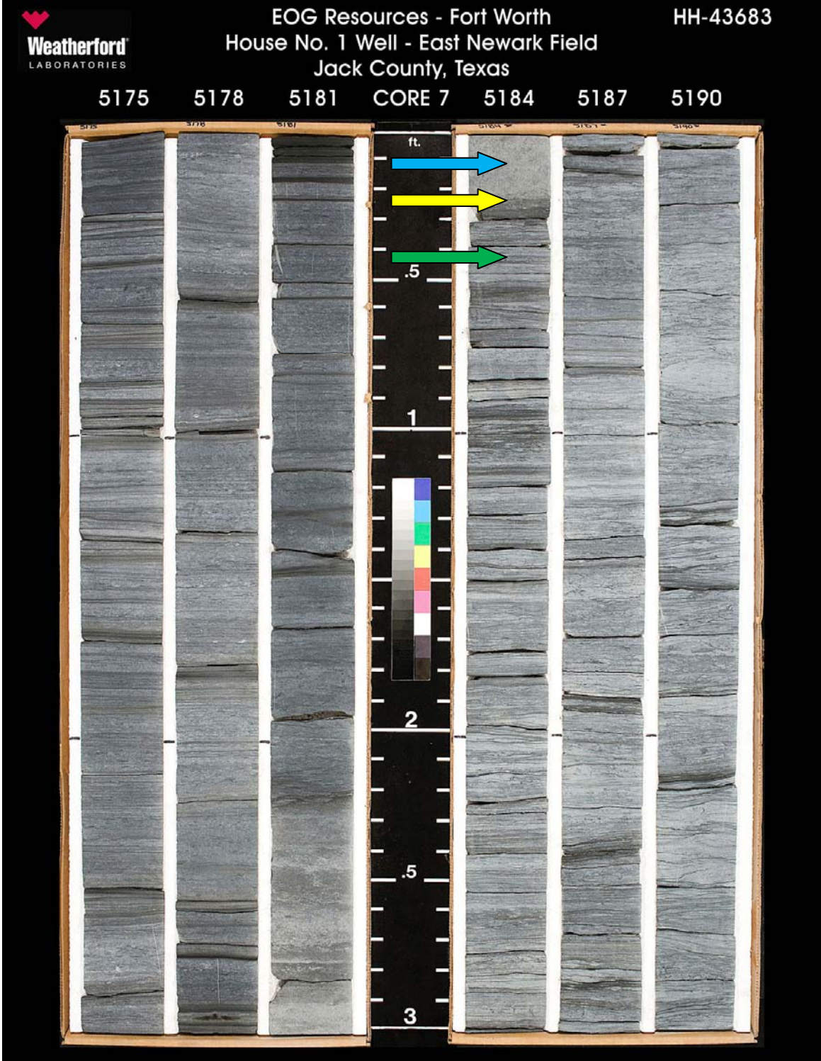
5175 - 5193 ft. Facies C and facies D. Note sharp contact (yellow arrow) between facies C (blue arrow) and D (green arrow). Also note wavy laminae of facies D.
