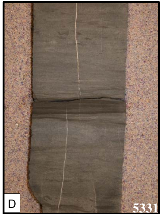
Figure 38. Core photos of fractures in Marble Falls clastic interval. Photo A and B are of facies A. Photo C is of facies B. Photo D is of facies G. Core is 8 cm wide.
