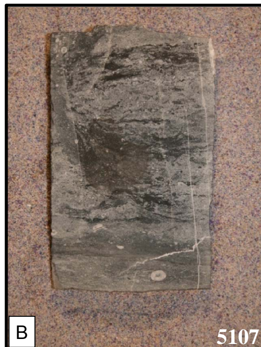
Figure 26. Core photos of facies B. Photo A shows claystone with thin interbeds of light gray spiculitic crinoidal siltstone. Photo B shows highly bioturbated light gray spiculitic crinoidal siltstone. Red outline indicates point at which Figure 27 was taken. Core is 8 cm wide.
