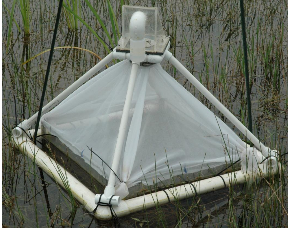
Figure 2. Photo of an emergence traps deployed on a pond. The net had a mesh size of 1.5mm.
