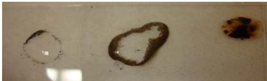
Figure 36. Optical images of the PSi samples with different surface chemistry. Left: octyl-functionalized PSi; Center: as-prepared PSi; Right: oxidized PSi.
