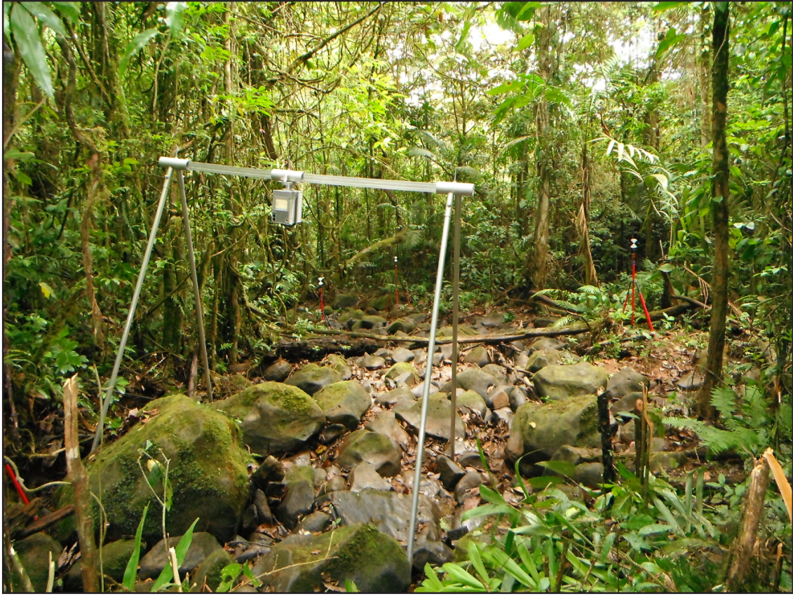
Figure 4. Terrestrial Laser Scanning (TLS) and target locations in reach A, looking downstream.
