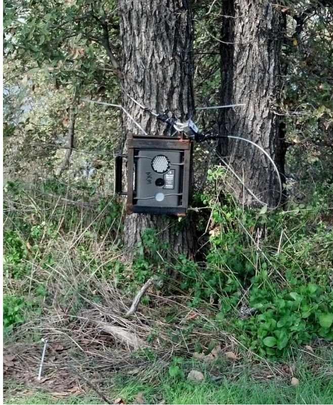
Figure 2. Photograph showing the security measures used with each camera.
