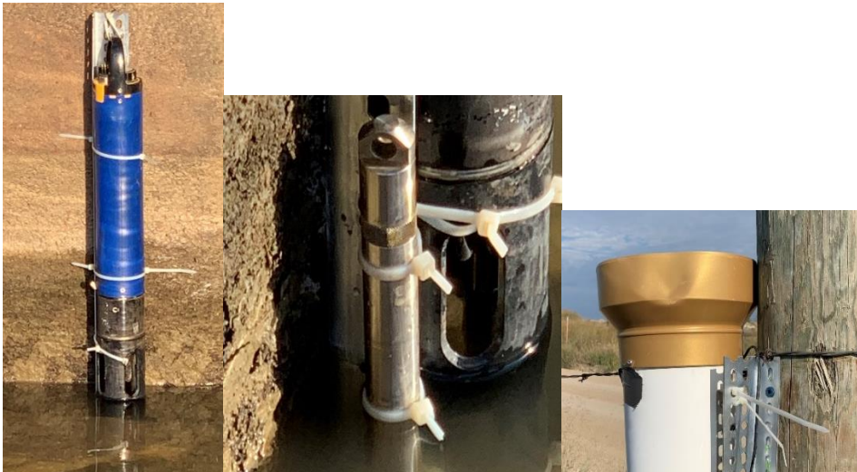
Figure 7: Continuous Monitoring Equipment. YSI EX01 Sonde (Left), Keller DCX-22 water level Data Logger (Middle), and RG 600 Tipping Bucket Rain Gauge (Right)
